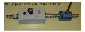
I don't know how much power the sampler will handle. I tried it on 20 meters running 150 Watts and it worked OK. I wouldn't try this one I built at a KW.
